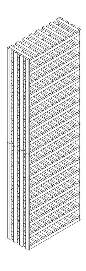
6. Anchor the racks to the wall using the recommended hardwares (not provided)
